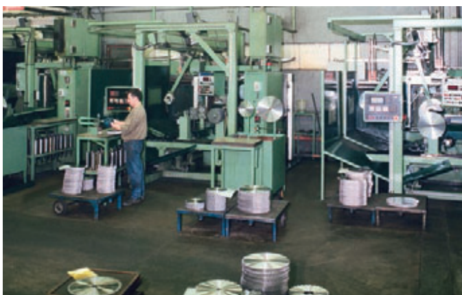
Grinding and tensioning the blades.
